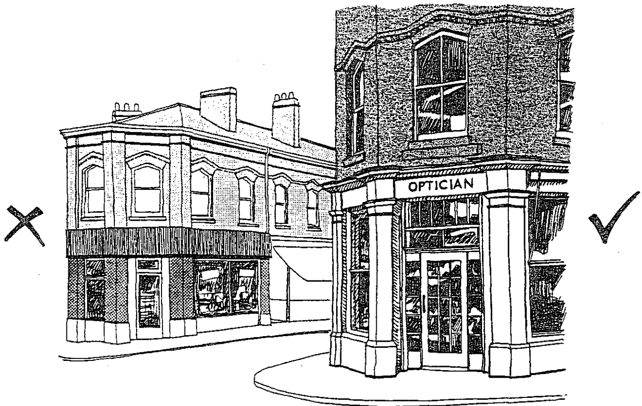
Fig. 5 One fascia sign (optician) carefully designed to retain the building details. In the other, opposite, all the details at the above ground floor have been obliterated by an oversized fascia and facing materials completely out of character with the building and the area.
