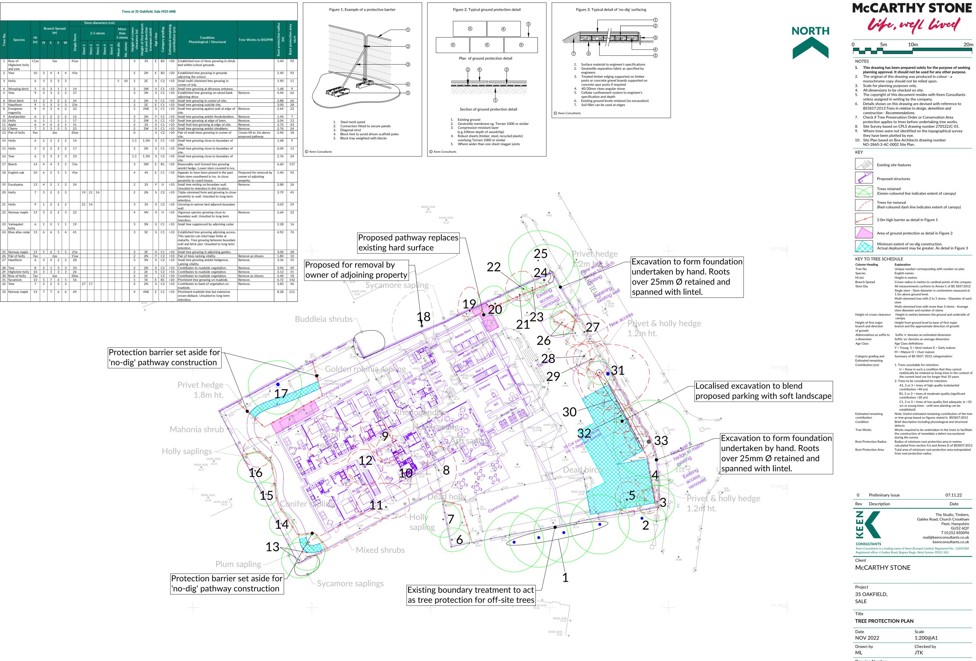
1. This drawing has been prepared solely for the purpose of seeking
