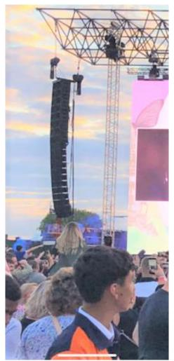
2.22. The front of the cabinets forming the stage right side hang was not visible from the measurement location adjacent to the site boundary. Consequently, turning the cabinets further away from the measurement location would be unlikely to reduce the levels at the survey position as this point was not in the direct "line of fire" of the line array i.e. in the zone with the highest levels from the PA.
