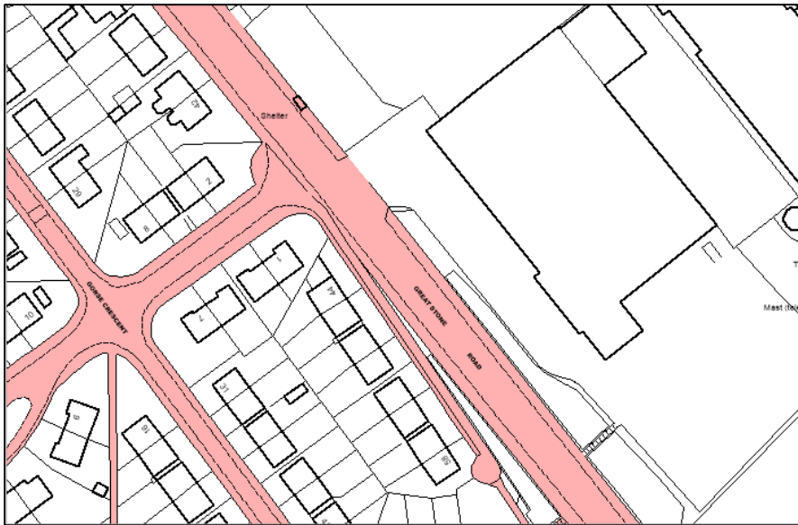
Figure 1 Extent of Adopted Highway (provided by Trafford Council)
