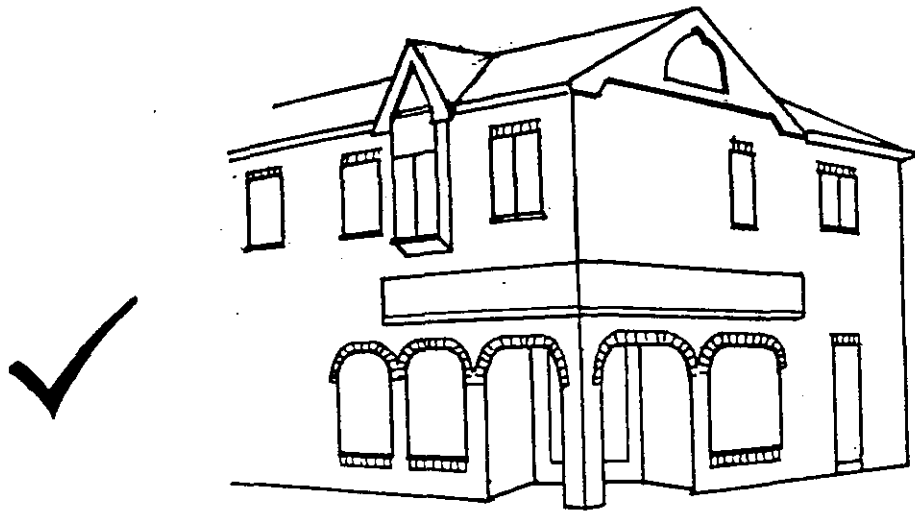
Shop front designed as an integral part of the building.
