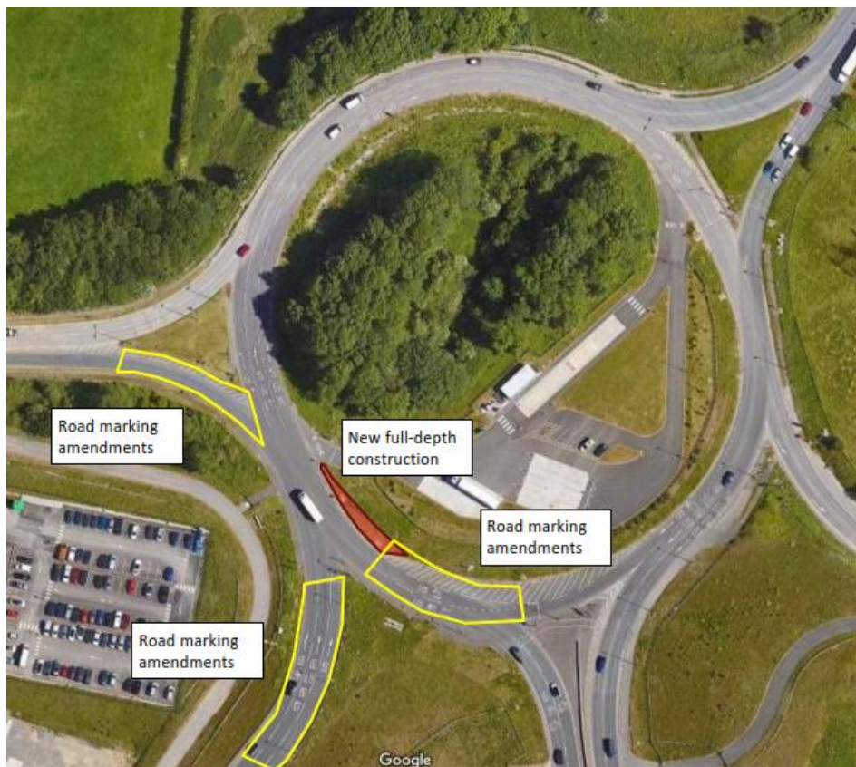
Figure 2.13 - WH8 - M56 Bowden roundabout, carriageway widening
