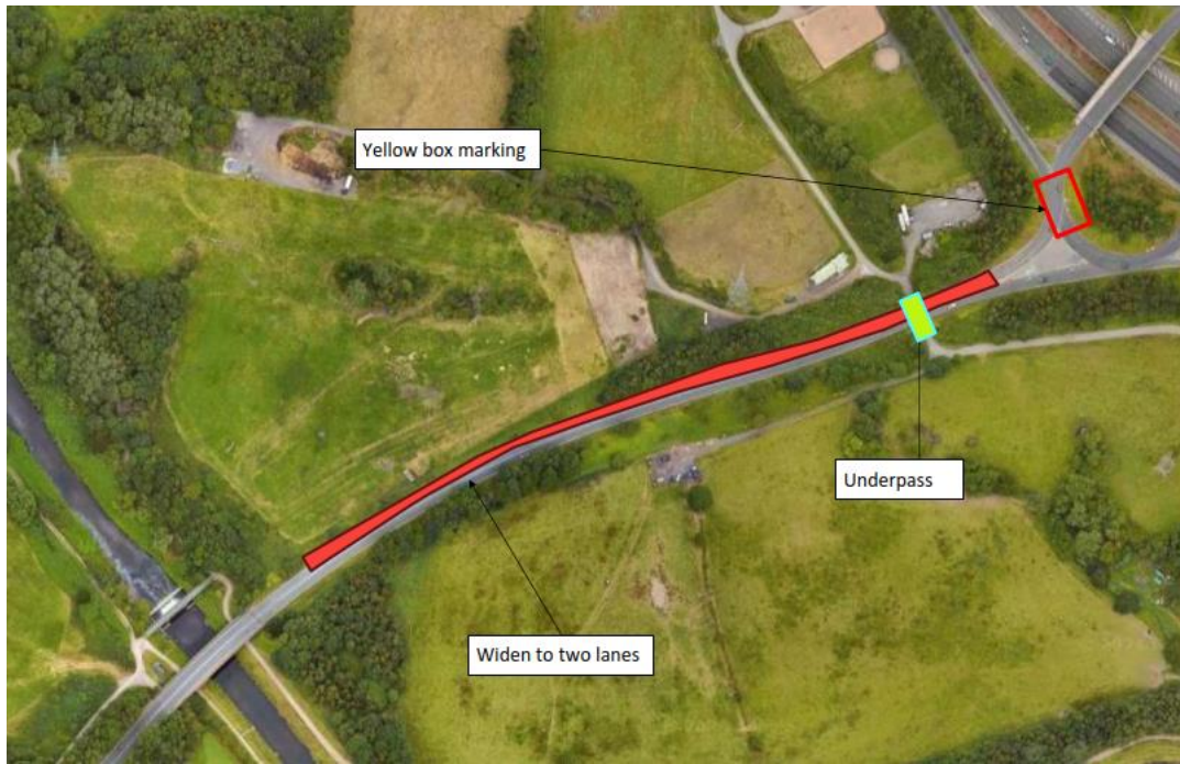
Figure 2.10 - WH3 - Carrington Spur widening eastbound to M60 J8
