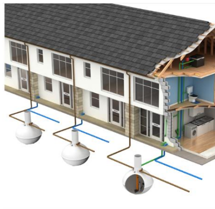
Photograph 48 - Example of Rainwater Harvesting
