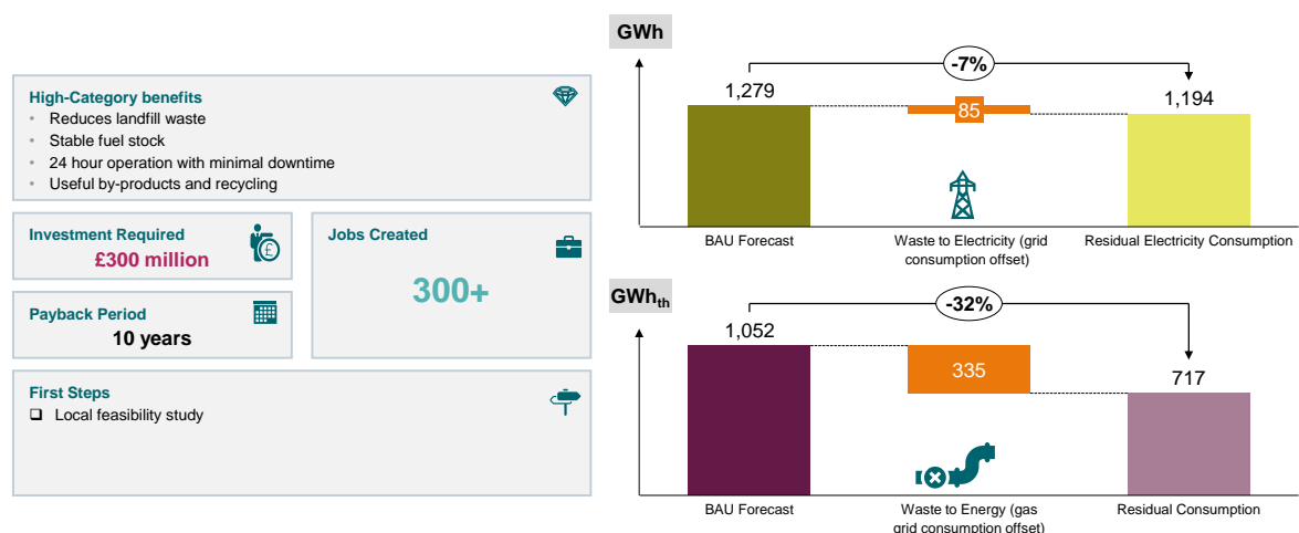
Figure 26: Key figures for a Waste to Energy facility generating 335 GWh th of heat, and 85 GWh of electricity per year
