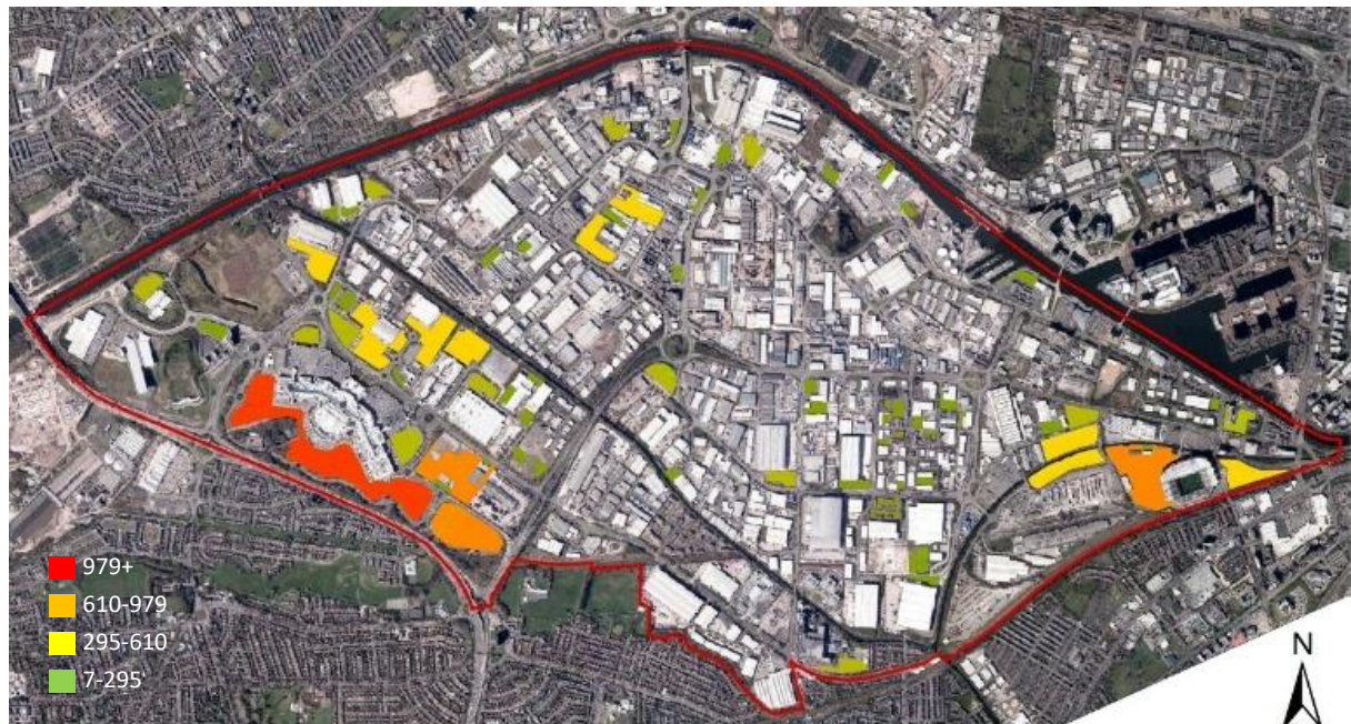
Figure 19: Solar Generation Car Port potential (MWh / year)
