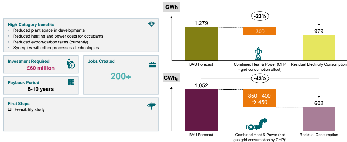
Figure 27: Key figures for CHP developments generating 400 GWh th of heat, and 300 GWh of electricity per year
