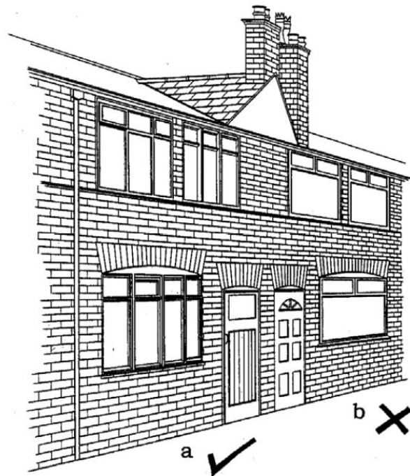
Examples of style five original doors and windows (left) and inappropriate replacements (right)
