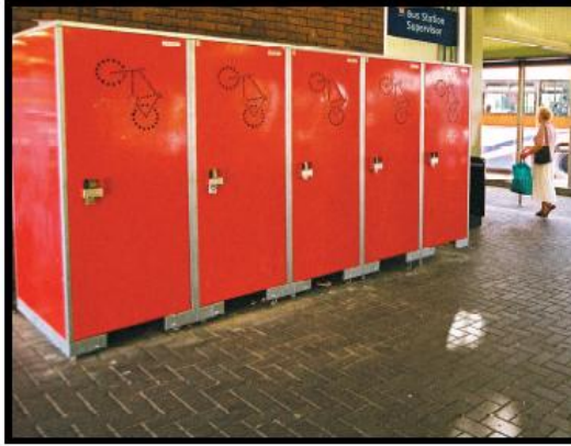
Fig 5: Vertical lockers are also considered unsuitable, since they cannot be used by some types of bicycle, and require lifting of the bicycle
